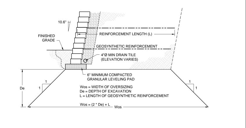
Drawn by: Scale: **ANCHOR**<sup>®</sup> Highland Stone® Retaining Wall System This drawing is for illustrative 3/8" = 1'-0" SB purposes only and should not be BUILD SOMETHING BEAUTIFUL used for construction without the Date: Drawing number: signature of a registered Typical Excavation Oversizing Cross Section © 2015 Anchor Wall Engineering, LLC HIRE08 professional engineer. ----® and <sup>™</sup> Anchor Wall Systems, Inc. www.anchorwall.com
