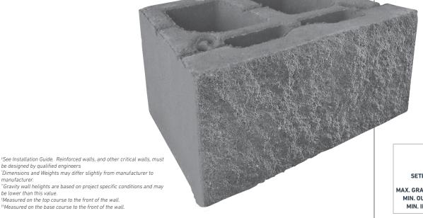
H X W X D' 8" X 18" X 12" WEIGHT' 75 LBS. COVERAGE 1 SQ. FT. 1" PER COURSE; 7.1° OR NEAR VERTICAL SETBACK & BATTER MAX. GRAVITY WALL HT." 4 FT. MIN. OUTSIDE RADIUS<sup>†</sup> 4 FT. MIN. INSIDE RADIUS<sup>††</sup> 6 FT.
