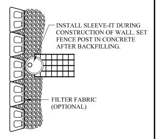
\*FENCING SYSTEMS APPROVED FOR USE WITH SLEEVE-IT ARE LIMITED TO THE FOLLOWING HEIGHTS: CHAIN LINK - UP TO 8-FT, PRIVACY - UP TO 6-FT (WOODEN, PVC, METAL). POST SIZE 4"X4" MAX.
