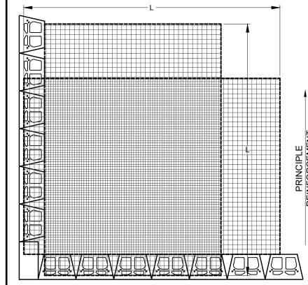
NOTE: USE ADHESIVE ON EXPOSED PARTIAL UNITS CUT UNITS (X) TO MAINTAIN RUNNING BOND
