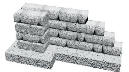
For the second course, center a medium stretcher unit over the base units as shown. Split another unit to maintain a staggered bond. Round the split ends with a hammer and chisel. Glue all units in the column with a concrete adhesive.
