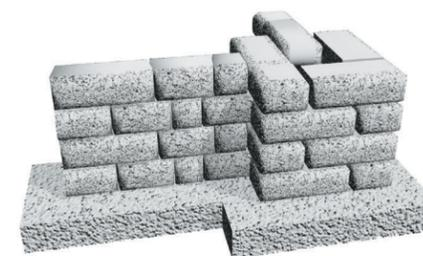
Frequently, a 90° turn is made at a column. To build this column, cut one column unit per course. Stack column units in a rotating pattern for each course. Glue each course of column units with a concrete adhesive.
