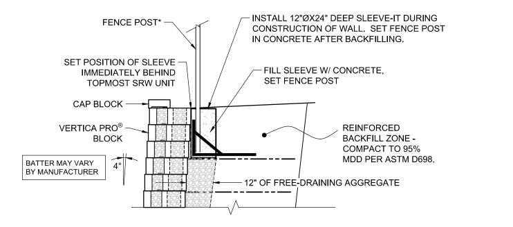
Scale: Drawn by: ANCHOR® Vertica Pro® Straight Face Retaining Wall System This drawing is for illustrative 3/8" = 1'-0" LM purposes only and should not be BUILD SOMETHING BEAUTIFUI used for construction without the Date: Drawing number signature of a registered © 2015 Anchor Wall Engineering, LLC Fence Section with Sleeve-It VPST10 professional engineer. ----® and <sup>™</sup> Anchor Wall Systems, Inc. www.anchorwall.com
