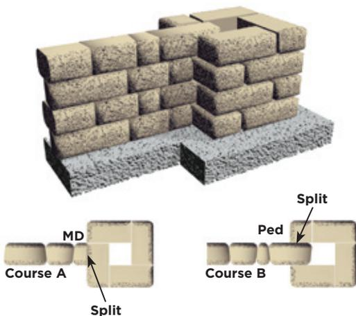
*\*To split a block, use a hydraulic splitter or split manually by using a hammer and chisel to score the block on all sides. Pound the chisel on the same line until the block splits. If partial unit sides are not exposed, use a circular cut-off saw with a masonry blade to achieve a tighter fit.*
