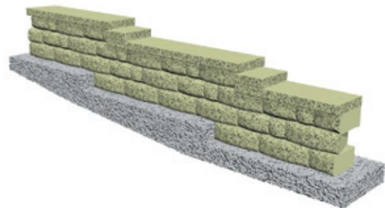
*\*To split a block, use a hydraulic splitter or split manually by using a hammer and chisel to score the block on all sides. Pound the chisel on the same line until the block splits. If partial unit sides are not exposed, use a circular cut-off saw with a masonry blade to achieve a tighter fit.*
