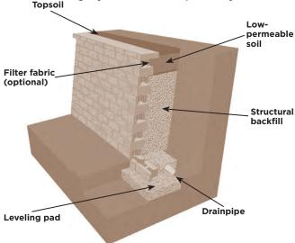
which offers a unique, nonconventional solution to problematic wall construction sites. It is a retaining wall built with Ancho products and self-compacting structural backfill specified by Anchor Wall Systems, and backed by engineering support tools developed by Anchor.
