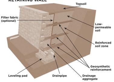
The second category is a geosynthetic-reinforced wall, which needs to be designed by a qualified engineer. There are (theoretically) no height
