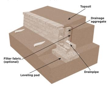
The first category – a gravity wall – is a retaining wall that does not use soil reinforcement. A gravity wall has height limitations specific to each product. An advantage of this type of retaining wall is that it requires a smaller work area behind the wall. A gravity wall relies on the weight and setback of the block to resist the soil forces being exerted on the wall.
