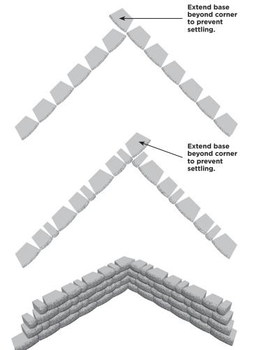
A quiet corner is sheltered with an inside 90° corner built with the Highland Stone® retaining wall system. Step up the caps in 3-inch increments for a finished look
