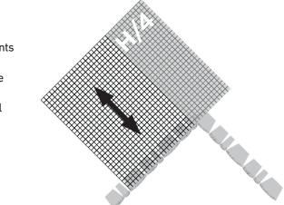
Alternate the geosynthetic reinforcement extension on each course where geogrid is required.
