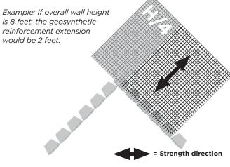
Place the next section of geogrid on the adjoining wall. The geogrid should not overlap and should lie flush with previously placed sections. Once geogrid is in place, the next courses of block can be installed.
