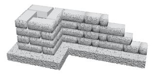
To build a column at the end of a wall, stack three column units as shown for the base course. For the second course, use column units, stacking in a rotating pattern. Glue each course of units in the column with concrete adhesive.
