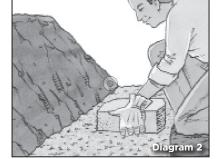
\*The Torpedo® base block is an option for Anchor freestanding walls instead of the large freestanding wall units.
