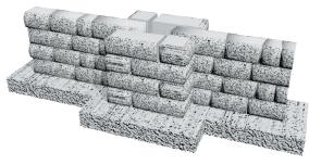
On the first course, use complete column units to start the column and cut the wall units to fit. On the second course, cut two column units in half to fill in the corners. Continue construction by alternating courses. Glue all column courses with a concrete adhesive.
