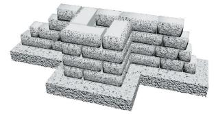
Columns add stability and elegance to a wall. They are located on one side of a wall. To build a column, stack column units in a rotating pattern for each course. Cut wall units as indicated. Glue each course of units in the column with a concrete adhesive.
