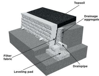
The first category - a gravity wall - is a retaining wall that does not use soil reinforcement. A gravity wall has height limitations specific to each product. An advantage of this type of retaining wall is that it requires a smaller work area behind the wall. A gravity wall relies on the weight and setback of the block to resist the soil forces being exerted
