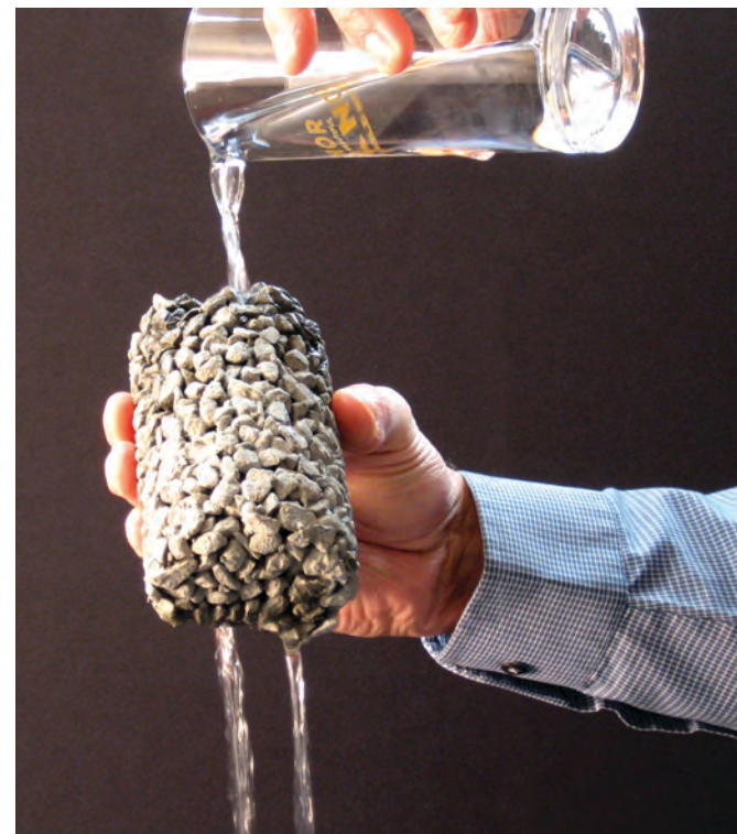
The structural backfill that meets Anchor Wall Systems, Inc.'s specifications allows water to drain behind the wall.
